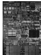
PowerPC® 940 (G5) 58M transistors / 2GHz / 97W L=0.13µm Area=118mm 2
